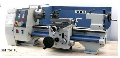
A reversible 2-mm pitch lead screw provides extended threading capability. You can create every American Standard Unified class 2A inch screw thread from 8 to 80 threads per inch, and you can create every American Standard Metric class 6h thread from 0.2 to 8 mm pitch with the change gears that are included.
